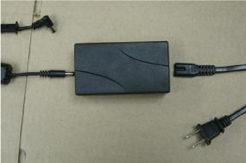
Figure 5 – How the power pack should be assembled
